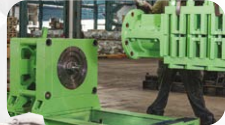
CLAMPING BAR CAGE ADAPTABLE TO EVERY MACHINE HOUSING & BASE FRAME
