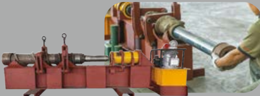
QUICK REPLACEMENT WITH HYDRAULIC JACK WORM AND COLLAR
