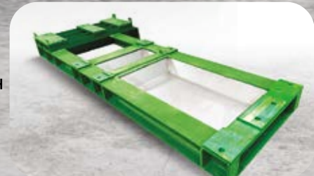
DUO-OIL PAN IS USED TO SEGREGATE PKO AND MINERAL OIL
