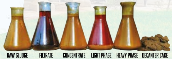
RAW SLUDGE FILTRATE CONCENTRATE LIGHT PHASE HEAVY PHASE DECANTER CAKE
