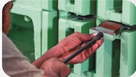
DETACHABLE INDIVIDUAL SLOT BLADE FEATURES TO EMPOWER MAINTENANCE DOWNTIME
