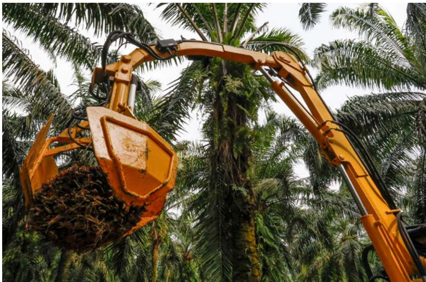
An autonomous mechanical buffalo grabber at the SD Guthrie palm oil plantations in Selangor. (Photo: Samsul Said/Bloomberg) (Bloomberg)
